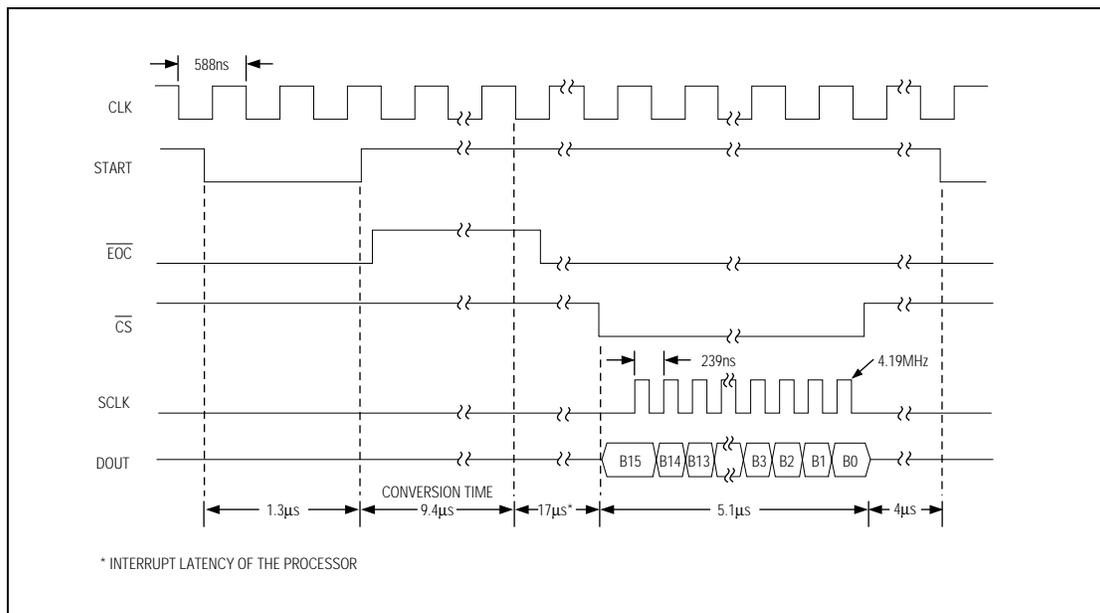
Figure 20. Timing Diagram for Circuit of Figure 19 (Mode 2)
