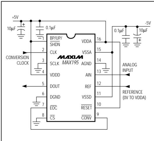
Figure 8. MAX1995 in the Simplest Operating Configuration
