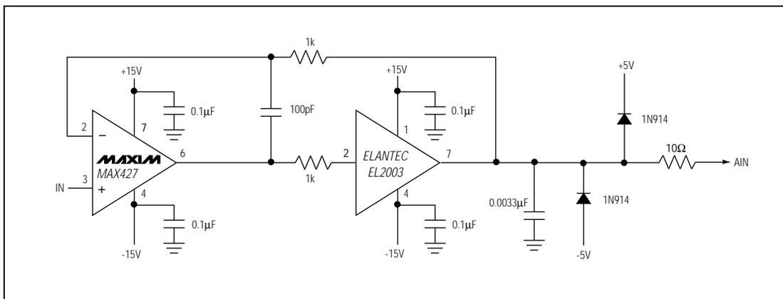
Figure 15. AIN Buffer for AC/DC Use
