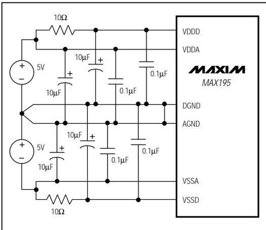
Figure 22. Supply Bypassing and Grounding
