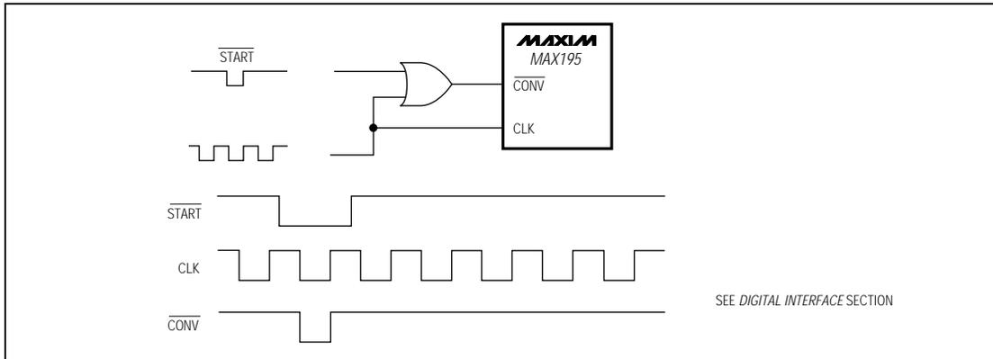
Figure 5. Gating  $\overline{\text{CONV}}$  to Synchronize with CLK
