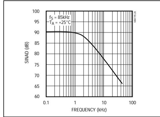
Figure 28. Signal-to-Noise + Distortion vs. Frequency
