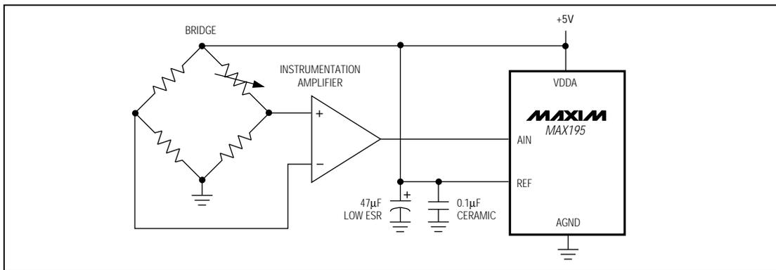
Figure 9. Ratiometric Measurement Without an Accurate Reference
