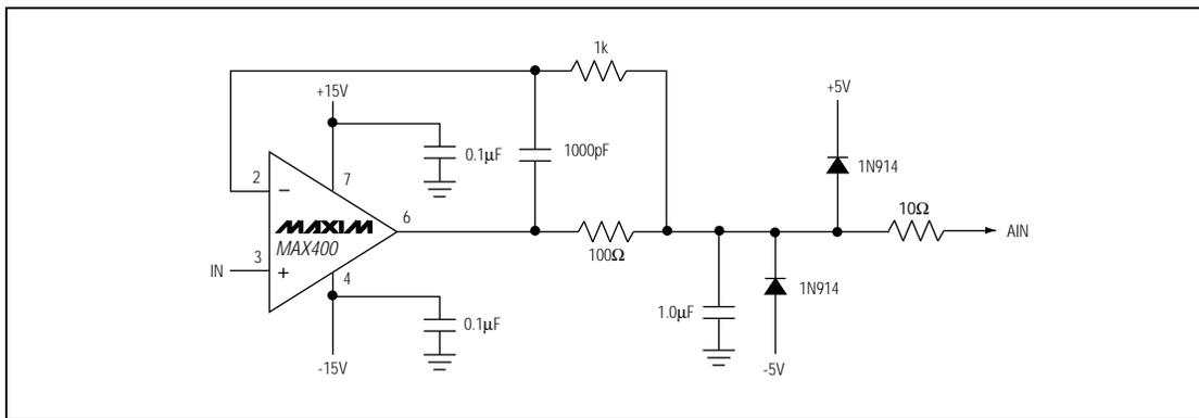
Figure 14. MAX400 Drives AIN for Low-Frequency Use
