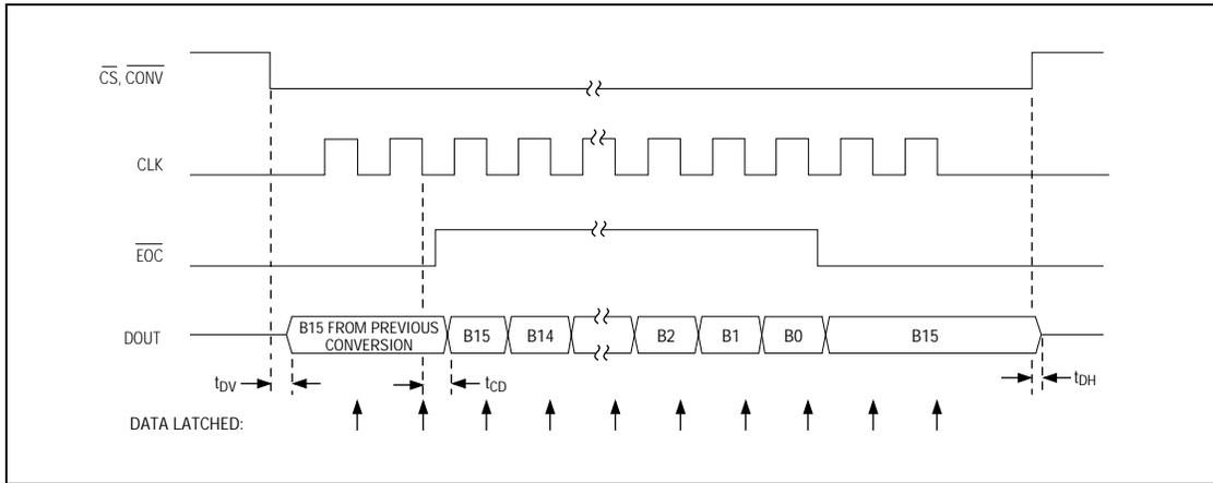
Figure 18. Timing Diagram for Circuit of Figure 17 (Mode 1)
