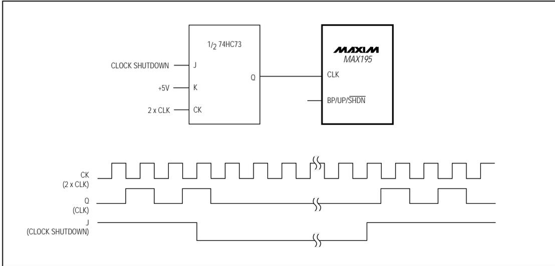
Figure 24. Circuit to Stop Free-Running Asynchronous CLK
