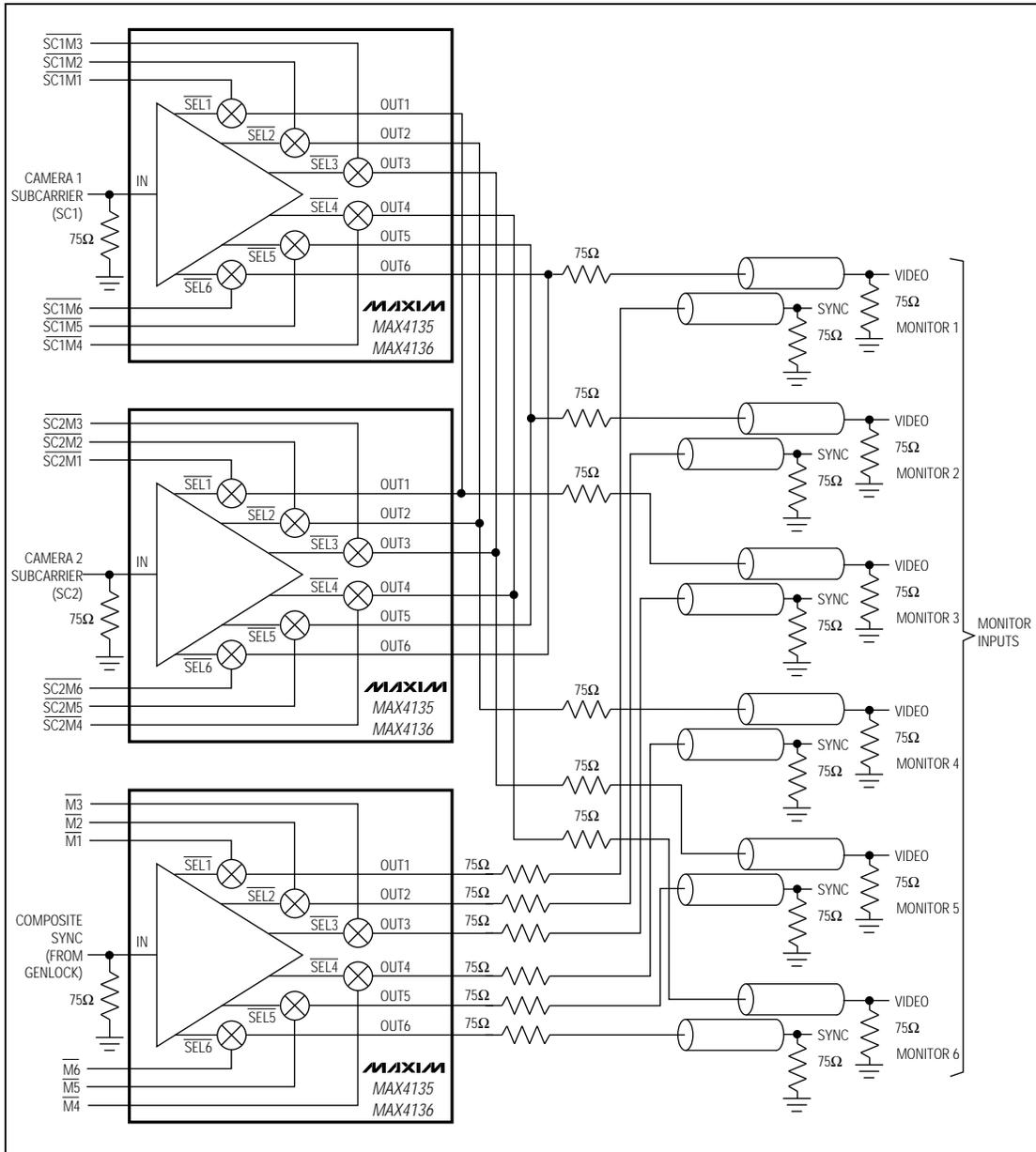
Figure 6. Two Cameras to Six Monitors Distribution Amplifier
