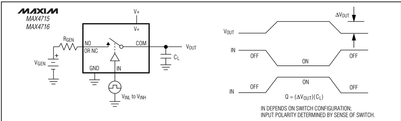
Figure 2. Charge Injection
