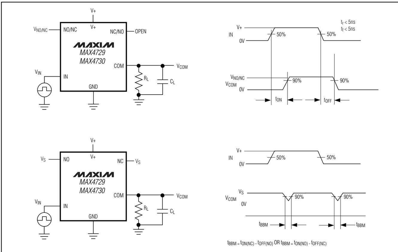
Figure 1. Switching Times
