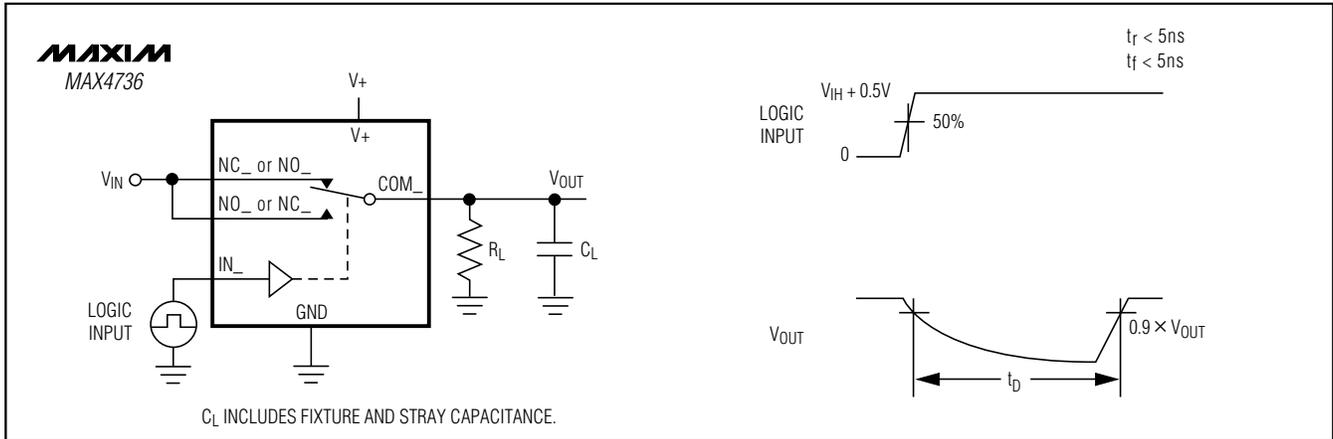
Figure 2. Break-Before-Make Interval
