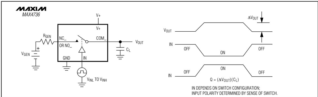
Figure 3. Charge Injection
