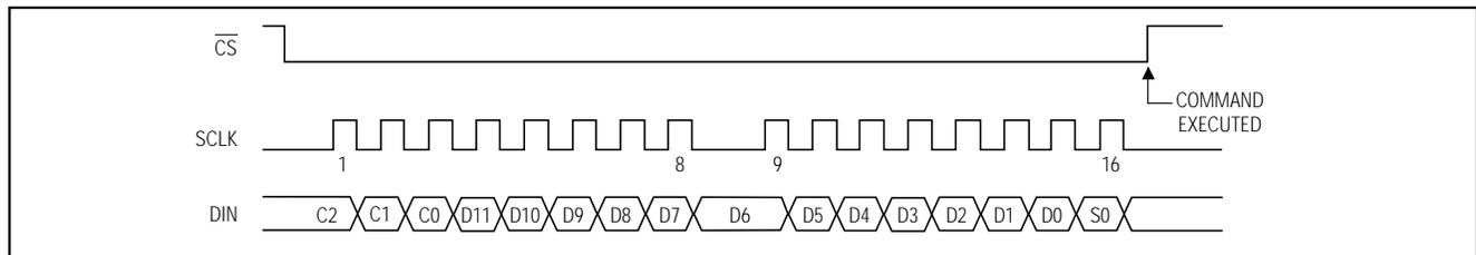
Figure 6. Serial-Interface Timing
