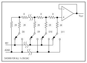
Figure 1. Simplified DAC Circuit Diagram
