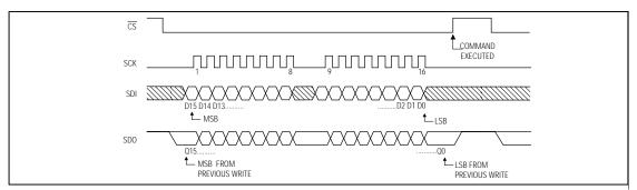
Figure 4. 3-Wire Serial-Interface Timing Diagram (LDAC = GND or VDD)
