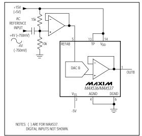
Figure 12. AC Reference Input Circuit
