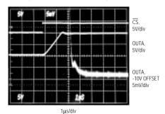
$V_{DD}$  = +15V,  $V_{SS}$  = -5V, REFAB = 10V,  $C_L$  = 100pF,  $R_L$  = 10k $\Omega$
