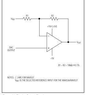
Figure 11. Bipolar Output Circuit
