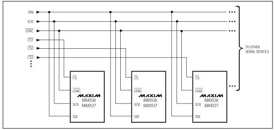
Figure 9. Multiple devices sharing a common DIN line may be simultaneously updated by bringing LDAC low. CS1, CS2, CS3... are driven separately, thus controlling which data are written to devices 1, 2, 3...
