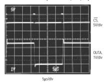
$V_{DD}$  = +5V,  $V_{SS}$  = -5V, REFAB = 2.5V,  $C_L$  = 100pF,  $R_L$  = 10k $\Omega$
