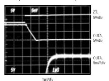
$V_{DD}$  = +15V,  $V_{SS}$  = -5V, REFAB = 10V,  $C_L$  = 100pF,  $R_L$  = 10k $\Omega$
