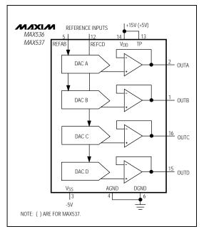
Figure 10. Unipolar Output Circuit
