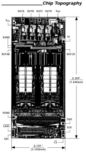
TRANSISTOR COUNT: 5034; SUBSTRATE CONNECTED TO VDD.
