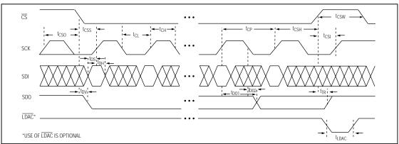
Figure 6. Detailed Serial-Interface Timing Diagram
