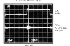
$\rm V_{DD}$  = +5V,  $\rm V_{SS}$  = -5V, REFAB = 2.5V,  $\overline{\rm CS}$  = HIGH, DIN TOGGLING AT  $^{1}\!\!/_{2}$  THE CLOCK RATE, OUTA = 1.25V
