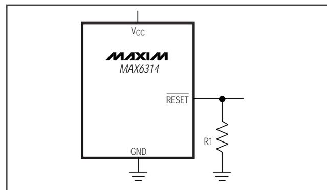
Figure 3.  $\overline{\text{RESET}}$  Valid to  $V_{\text{CC}} = \text{Ground}$  Circuit
