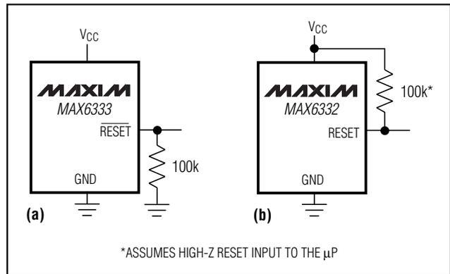
Figure 2. Ensuring Reset Valid Down to VCC = 0
