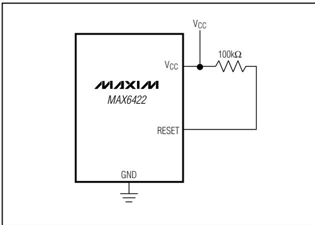
Figure 4. Ensuring RESET Valid to  $V_{CC} = 0$
