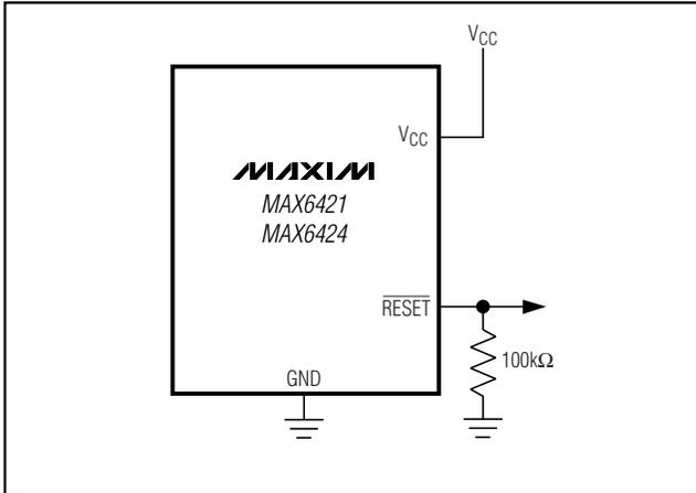
Figure 3. Ensuring RESET Valid to  $V_{CC} = 0$
