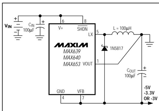
Figure 6. Inverting Configuration
