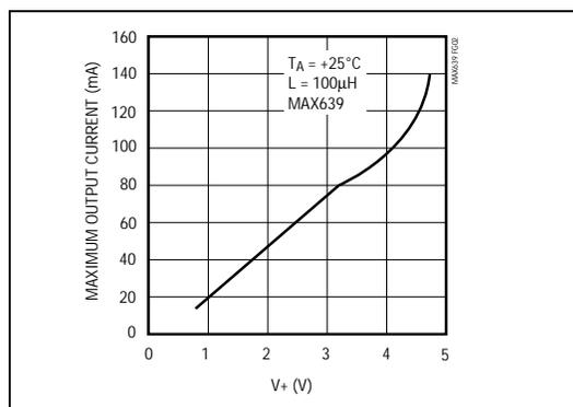
Figure 7. Maximum Current Capability of Figure 6 Circuit
