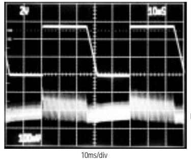
A:  $V_{IN}$ , 6V TO 11.5V, 2V/div
