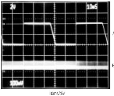
A:  $V_{IN}$ , 4V TO 8V, 2V/div
