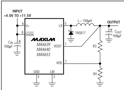
Figure 4. Adjustable-Output Operation
