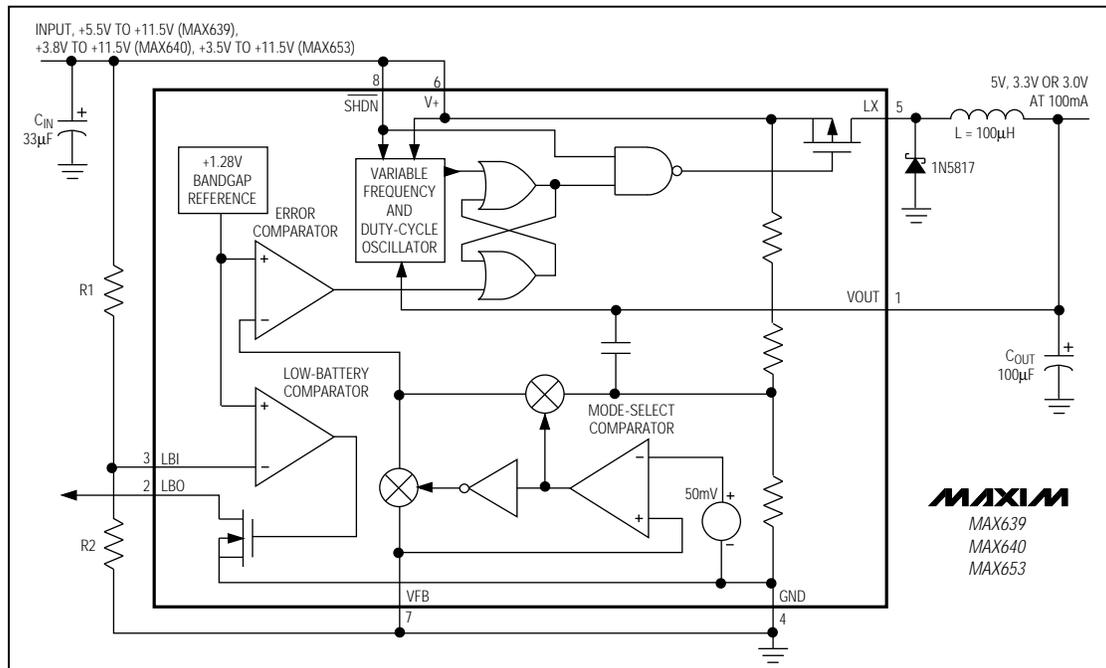
Figure 3. Block Diagram
