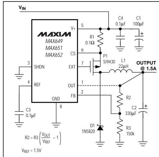
Figure 4. Adjustable-Output Operation
