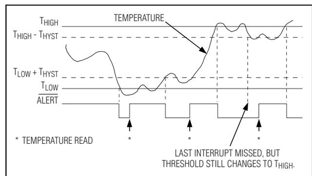
Figure 2. Example of  $\overline{\text{ALERT}}$  Operation in Interrupt Mode
