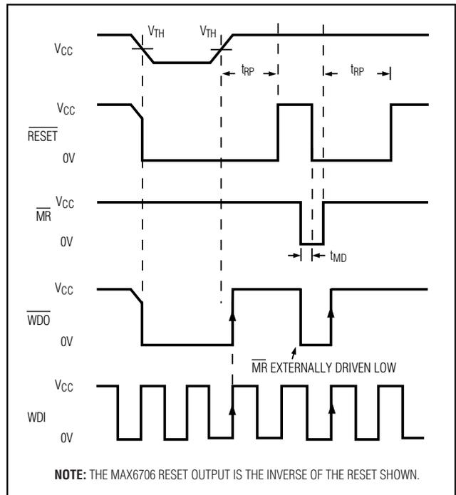
Figure 4. MAX6705/MAX6706/MAX6707  $\overline{\text{RESET}}$ ,  $\overline{\text{MR}}$ ,  $\overline{\text{WDO}}$ , and  $\overline{\text{WDI}}$  Timing
