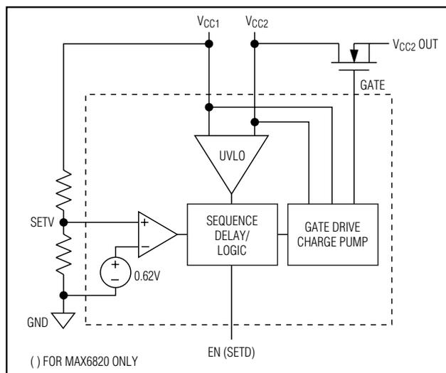
Figure 1. Functional Diagram
