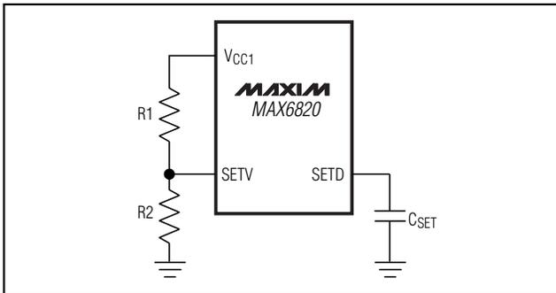
Figure 2.  $t_{DELAY}$  (MAX6820 ONLY) and  $V_{TH}$  Adjust
