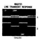
A: V<sub>OUT</sub>, 100mV/div B: V<sub>IN</sub>, 2V to 3V Circuit of Fig. 2a,  $I_{LOAD} = 200mA$  $T_A = +25^{\circ}C$
