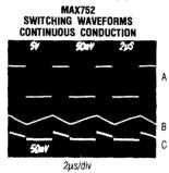
A: Switch Voltage (LX pin), 5V/div, 0V to +12.4V B: Inductor Current, 500mA/div C: Output Voltage Ripple, 50mV/div Circuit of Fig. 2b, Cout =  $300\mu$ F, V = 3V, Iout = 100mA, TA =  $+25^{\circ}$ C
