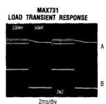
A: VOUT,100mV/div B:  $I_{OUT}$ , 100mA/divCircuit of Fig. 2a,  $T_A = +25^{\circ}C$
