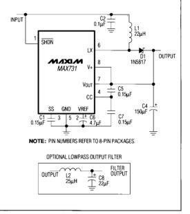
Figure 2a. MAX731 Standard Boost Application Circuit
