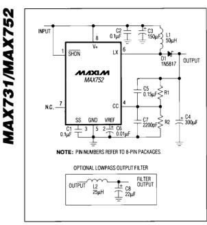
Figure 2b. MAX752 Standard Boost Application Circuit
