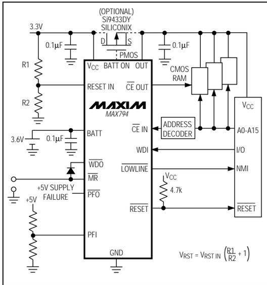
Figure 3. MAX794 Standard Application Circuit
