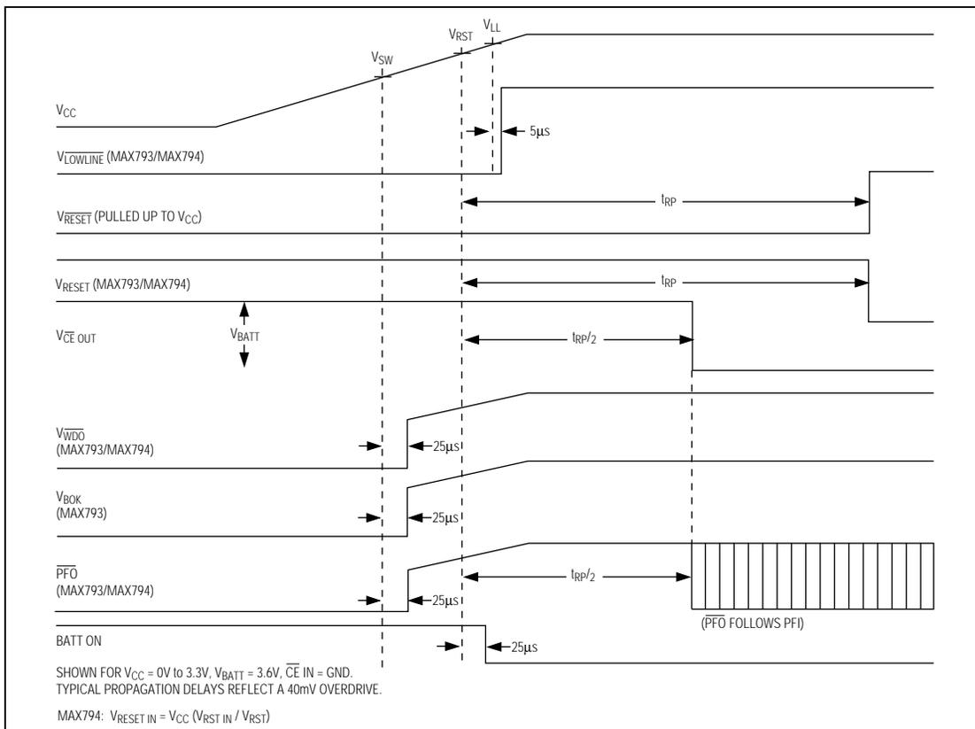
Figure 1. Timing Diagram,  $V_{CC}$  Rising
