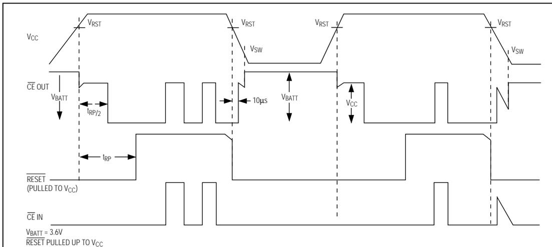
Figure 8. Chip-Enable Timing
