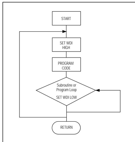
Figure 19. Watchdog Flow Diagram
