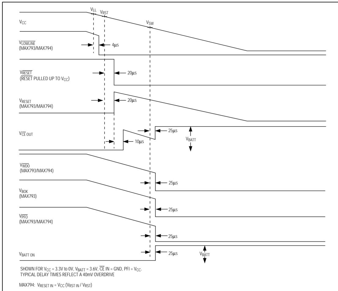
Figure 2. Timing Diagram,  $V_{CC}$  Falling
