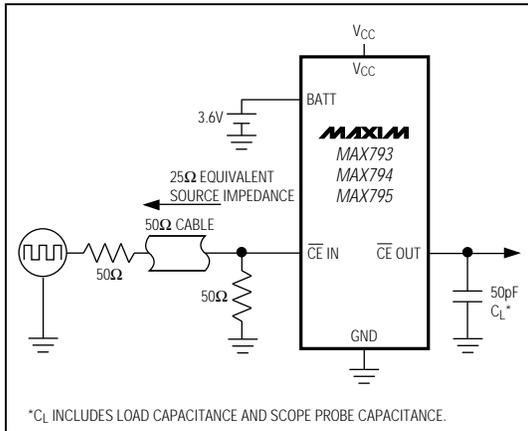
Figure 9. CE Propagation Delay Test Circuit
