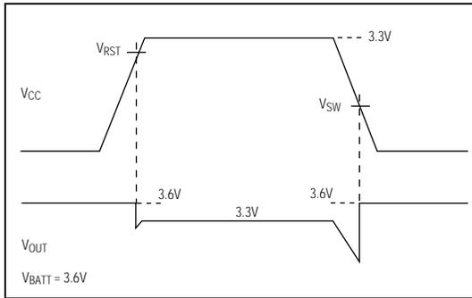
Figure 13. Battery Switchover Timing
