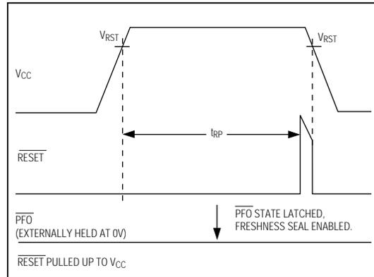
Figure 4. Battery Freshness Seal Enable Timing
