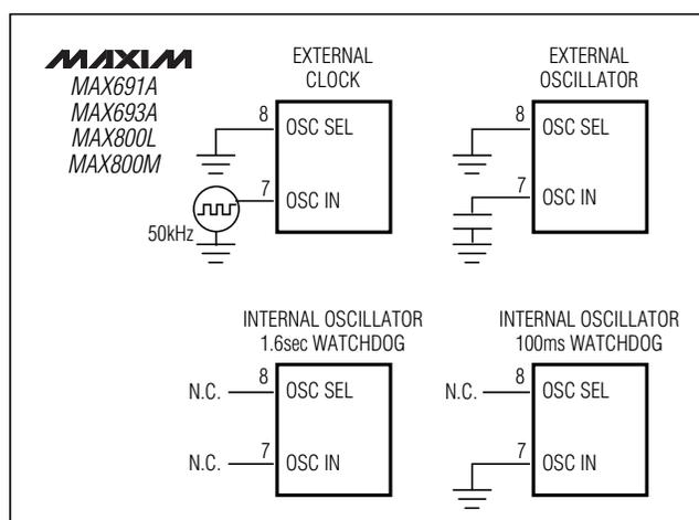
Figure 3. Oscillator Circuits
