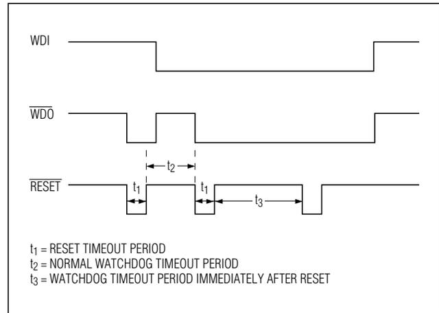
Figure 2. Watchdog Timeout Period and Reset Active Time
