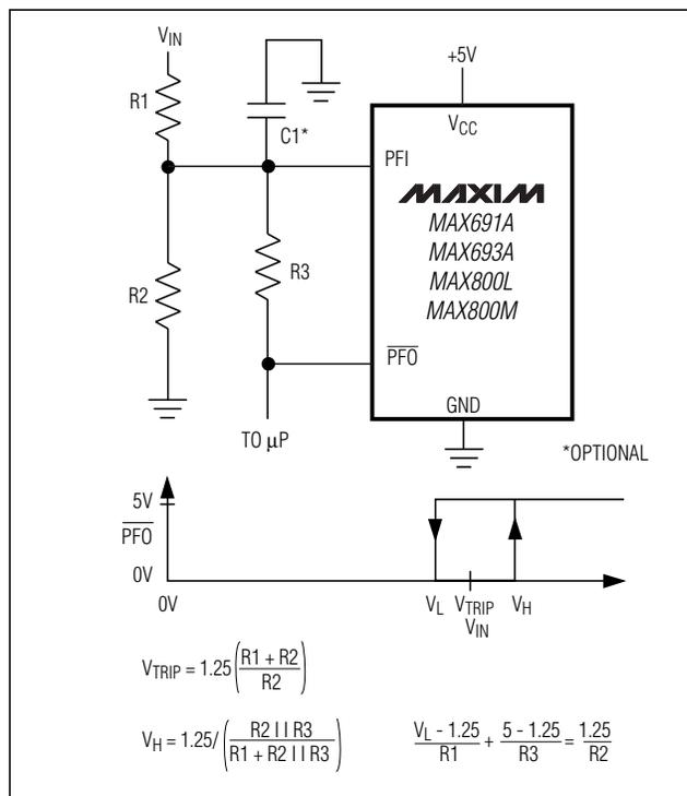
Figure 11. Adding Hysteresis to the Power-Fail Comparator
