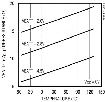
**V<sub>CC</sub> to V<sub>OUT</sub> ON-RESISTANCE vs. TEMPERATURE**
