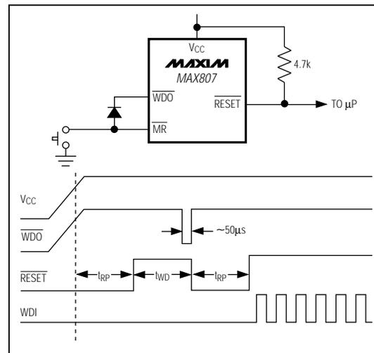
Figure 6. Generating a Reset on Each Watchdog Fault
