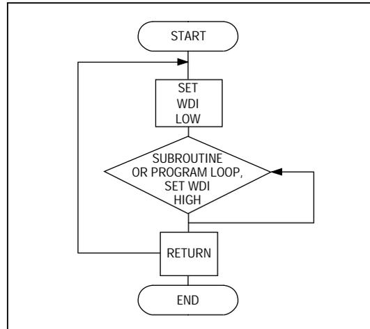
Figure 16. Watchdog Flow Diagram
