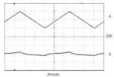
A: INPUT VOLTAGE, 2V/div, 2V to 4.5V B: OUTPUT VOLTAGE, 50mV/div MAX878L, I<sub>OUT</sub> = 100mA, V<sub>OUT</sub> = 3.3V
