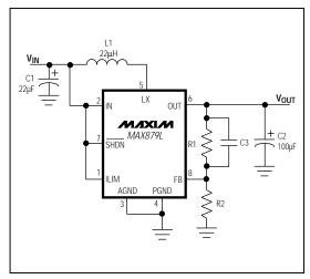
Figure 3. MAX879L Adjustable Voltage
