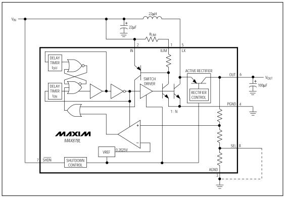
Figure 1. MAX878L Block Diagram
