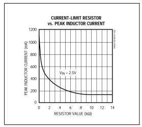
Figure 2. Current-Limit Resistor vs. Peak Inductor Current
