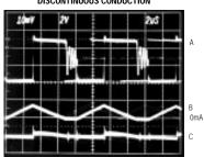
$\begin{array}{c} 2\mu s/\text{div} \\ \text{A: SWITCH VOLTAGE (LX PIN), } 2V/\text{div} \\ \text{B: INDUCTOR CURRENT, } 0.5A/\text{div} \\ \text{C: OUTPUT VOLTAGE RIPPLE, } 50mV/\text{div} \\ \text{MAX877L, } V_{\text{IN}} = 3V, I_{\text{OUT}} = 70\text{mA} \end{array}$
