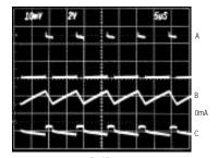
A: SWITCH VOLTAGE (LX PIN), 2V/div B: INDUCTOR CURRENT, 0.5A/div C: OUTPUT VOLTAGE RIPPLE, 50mV/div MAX877L, V<sub>IN</sub> = 1.5V, I<sub>OUT</sub> = 100mA
