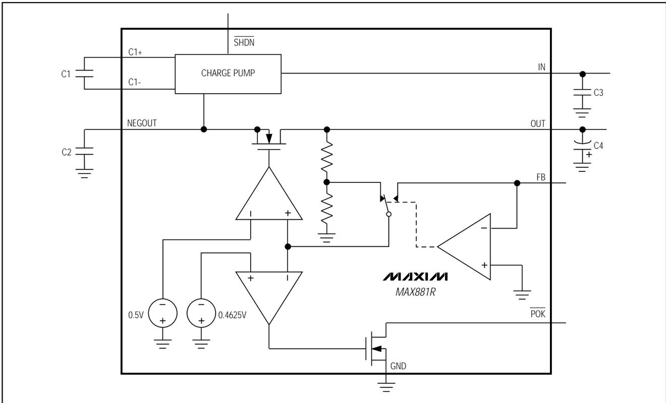
Figure 1. Functional Diagram
