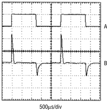
MAX883: V_{OUT} = 5V , C_{IN} = 0\mu F , t_R = 15\mu s , t_F = 13\mu s A: V_{IN} = 8V (HIGH) / V_{IN} = 7V (LOW) B: OUTPUT CURRENT (100mA/div)
