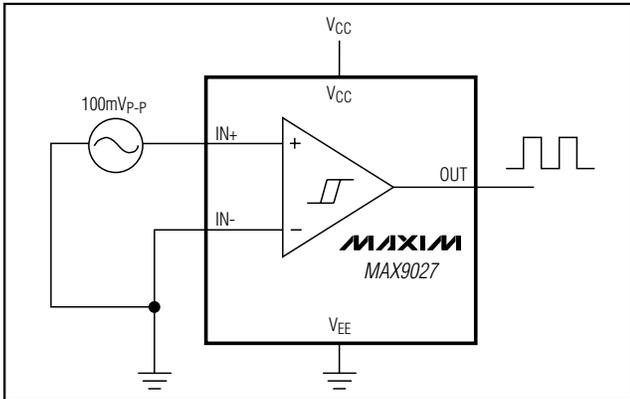
Figure 4. Zero-Crossing Detector
