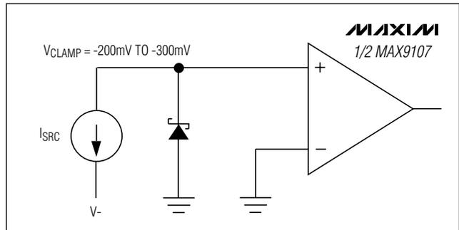
Figure 3. Schottky Clamp for Input Driven Below Ground
