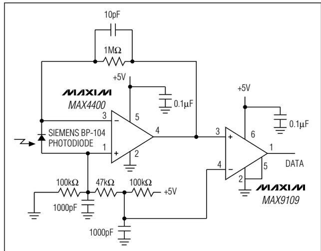
Figure 4. Battery-Operated Infrared Data Link Consumes Only 760µA
