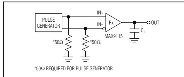
Figure 2. Propagation Delay and Transition Time Test Circuit
