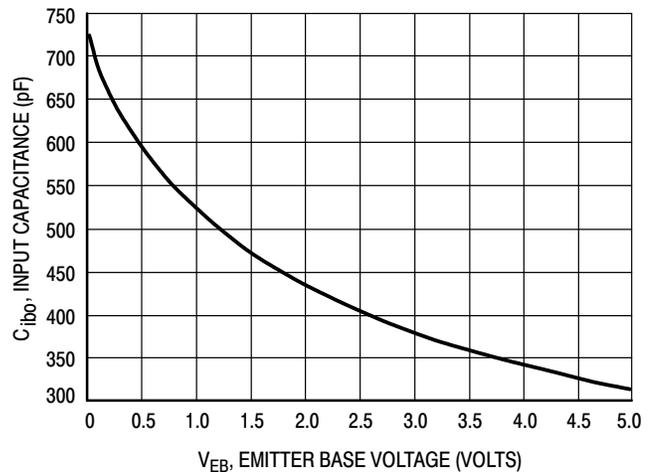
**Figure 6. Input Capacitance**
