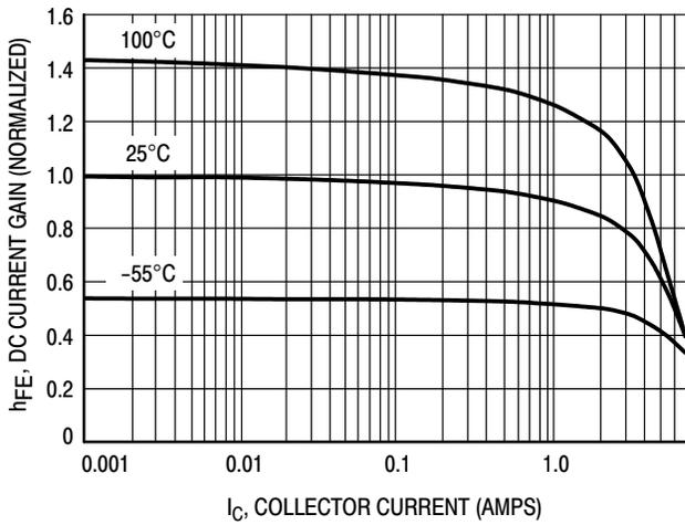
**Figure 3. DC Current Gain versus Collector Current**
