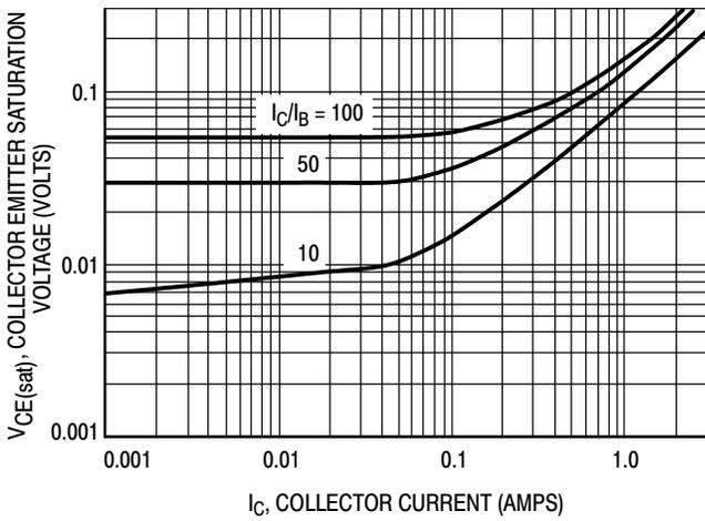
**Figure 1. Collector Emitter Saturation Voltage versus Collector Current**
