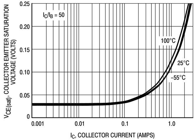
**Figure 2. Collector Emitter Saturation Voltage versus Collector Current**
