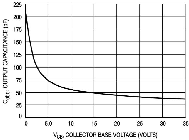
Figure 7. Output Capacitance
