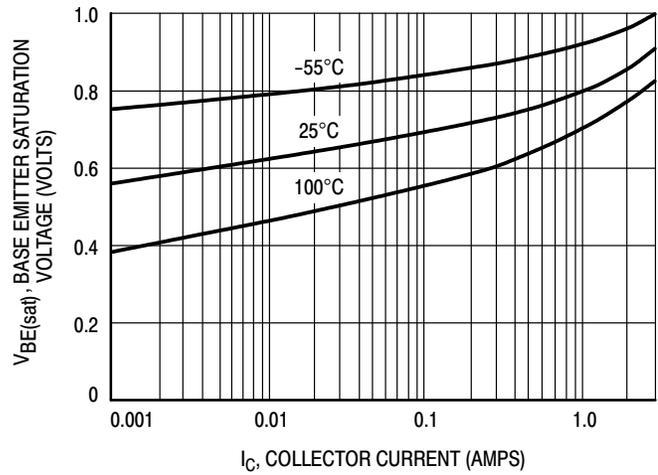
**Figure 4. Base Emitter Saturation Voltage versus Collector Current**
