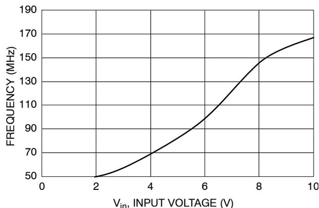
Figure 12. Plot 1. Dual Varactor MMBV609, V<sub>IN</sub> vs. Frequency
