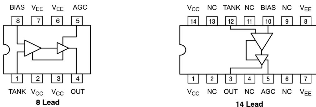
Warning: All  $V_{CC}$  and  $V_{EE}$  pins must be externally connected to Power Supply to guarantee proper operation.
