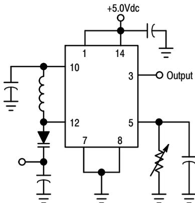
Figure 13. Method of Obtaining a Sine-Wave Output
