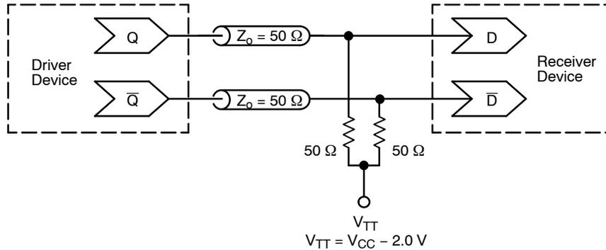
Figure 17. Typical Termination for Output Driver and Device Evaluation
