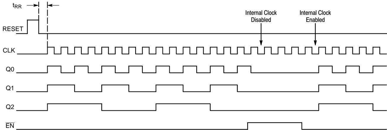
The  $\overline{\text{EN}}$  signal will freeze the internal clocks to the flip-flops on the first falling edge of CLK after its assertion. The internal dividers will maintain their state during the internal clock freeze and will return to clocking once the internal clocks are unfrozen. The outputs will transition to their next states in the same manner, time and relationship as they would have had the  $\overline{\text{EN}}$  signal not been asserted.
