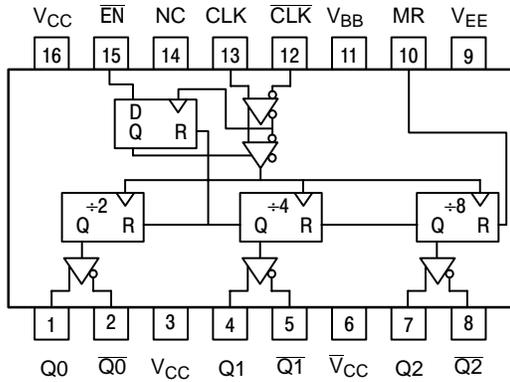
\* All  $V_{CC}$  pins are tied together on the die.
