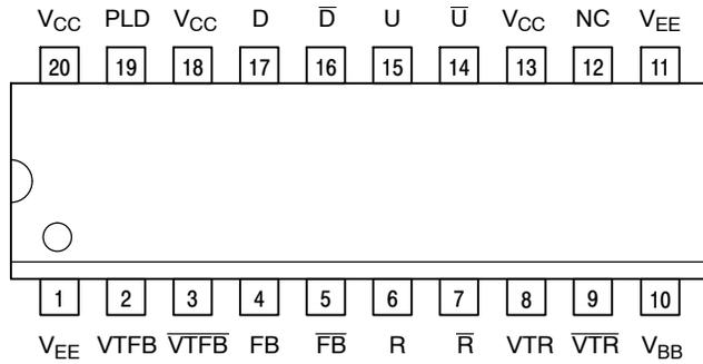
Warning: All V<sub>CC</sub> and V<sub>EE</sub> pins must be externally connected to Power Supply to guarantee proper operation.
