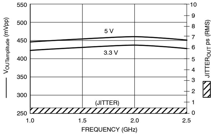
Figure 3. F<sub>max</sub>/Jitter @ 25°C
