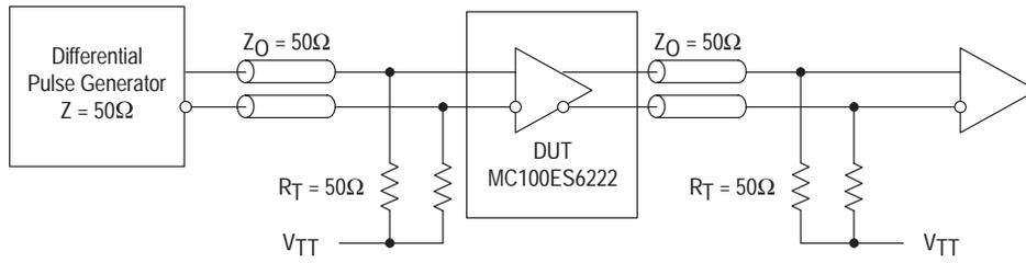
Figure 3. MC100ES6222 AC test reference
