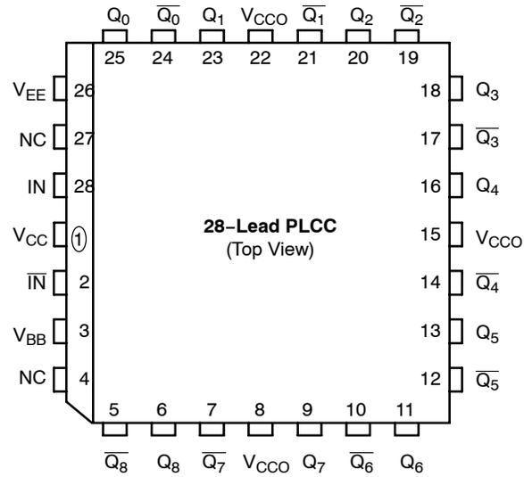
Warning: All  $V_{CC}$ ,  $V_{CCO}$ , and  $V_{EE}$  pins must be externally connected to Power Supply to guarantee proper operation.
