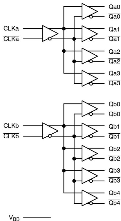
**Figure 2. Logic Diagram**
