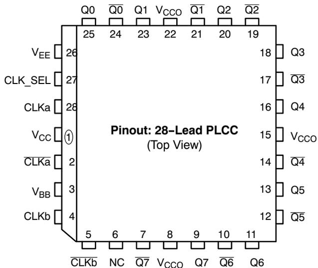
Warning: All  $V_{CC}$ ,  $V_{CCO}$ , and  $V_{EE}$  pins must be externally connected to Power Supply to guarantee proper operation.
