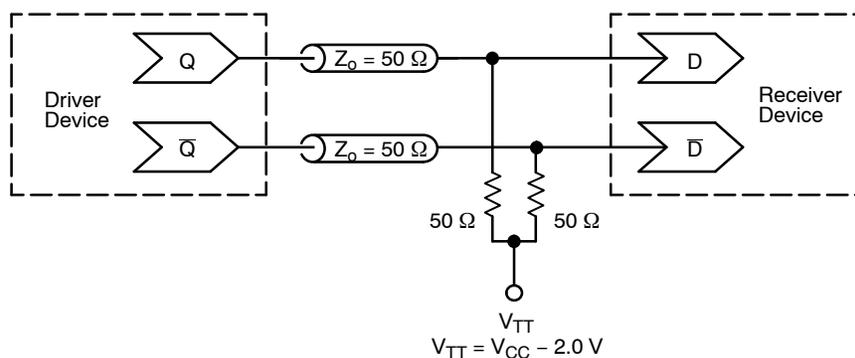
**Figure 2. Typical Termination for Output Driver and Device Evaluation**
