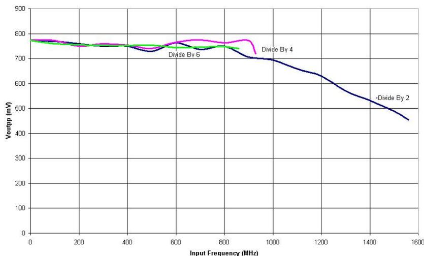
**Figure 4. Fmax: Voutpp vs Input Frequency per DIV2/4/6**
