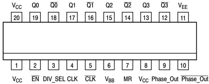
**Figure 1. Pinout: 20-Lead SOIC (Top View)**
