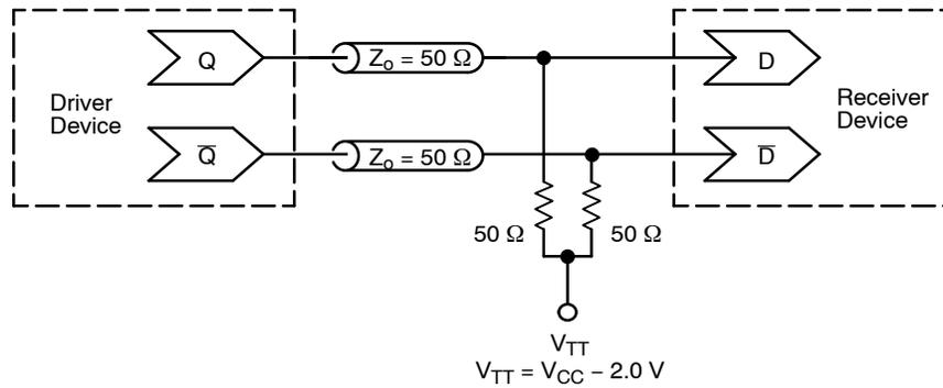
**Figure 5. Typical Termination for Output Driver and Device Evaluation
