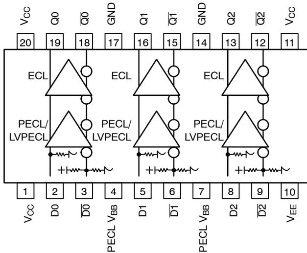
**Figure 1. SO-20 Pinout (Top View) and Logic Diagram**
