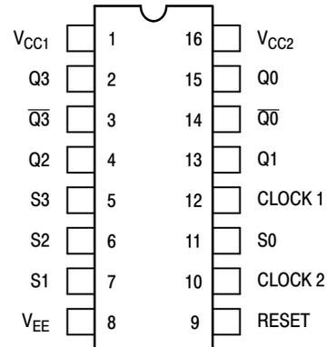
Pin assignment is for Dual-in-Line Package.
