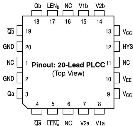
\* All V<sub>CC</sub> and V<sub>CC0</sub> pins are NOT tied together on the die.
