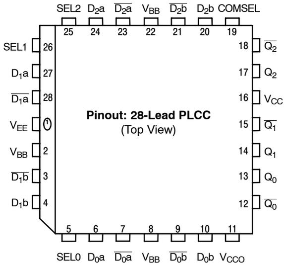
\* All  $V_{CC}$  and  $V_{CCO}$  pins are tied together on the die.
