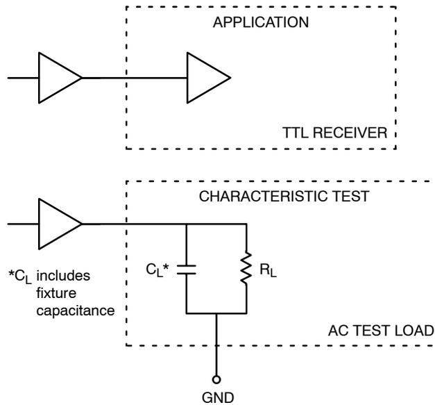
**Figure 2. TTL Output Loading Used for Device Evaluation**
