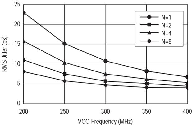
**Figure 8. RMS PLL Jitter versus VCO Frequency**
