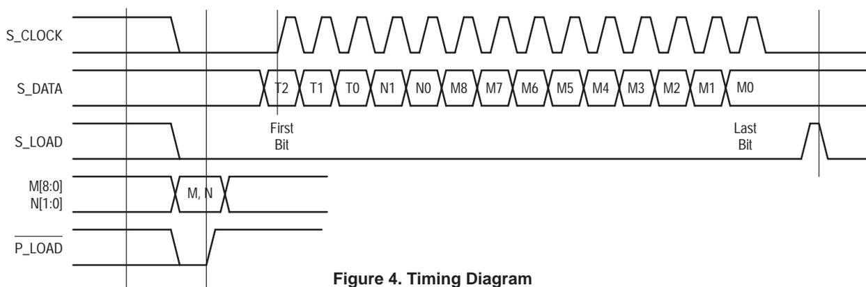
Figure 4. Timing Diagram
