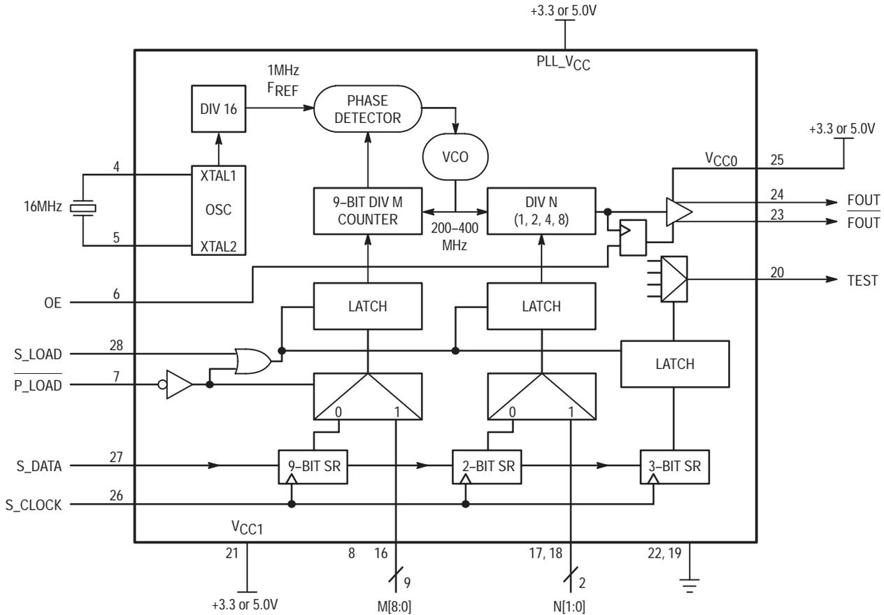
Figure 3. MC12429 Block Diagram (28-Lead PLCC Pinout)
