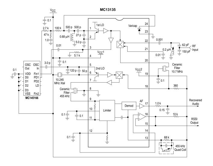
Figure 16. 144 MHz Single Channel Application Circuit
