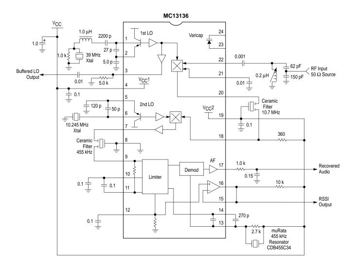
Figure 20b. Optional Audio Amplifier Circuit
