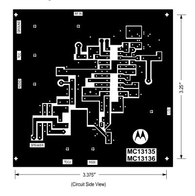
Figure 19. PC Board Component View
