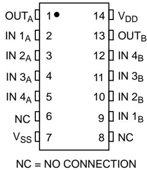
Figure 1. Pin Assignment
