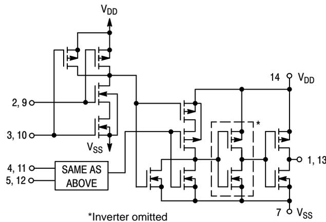
Figure 4. Circuit Schematic - One of Two Gates Shown
