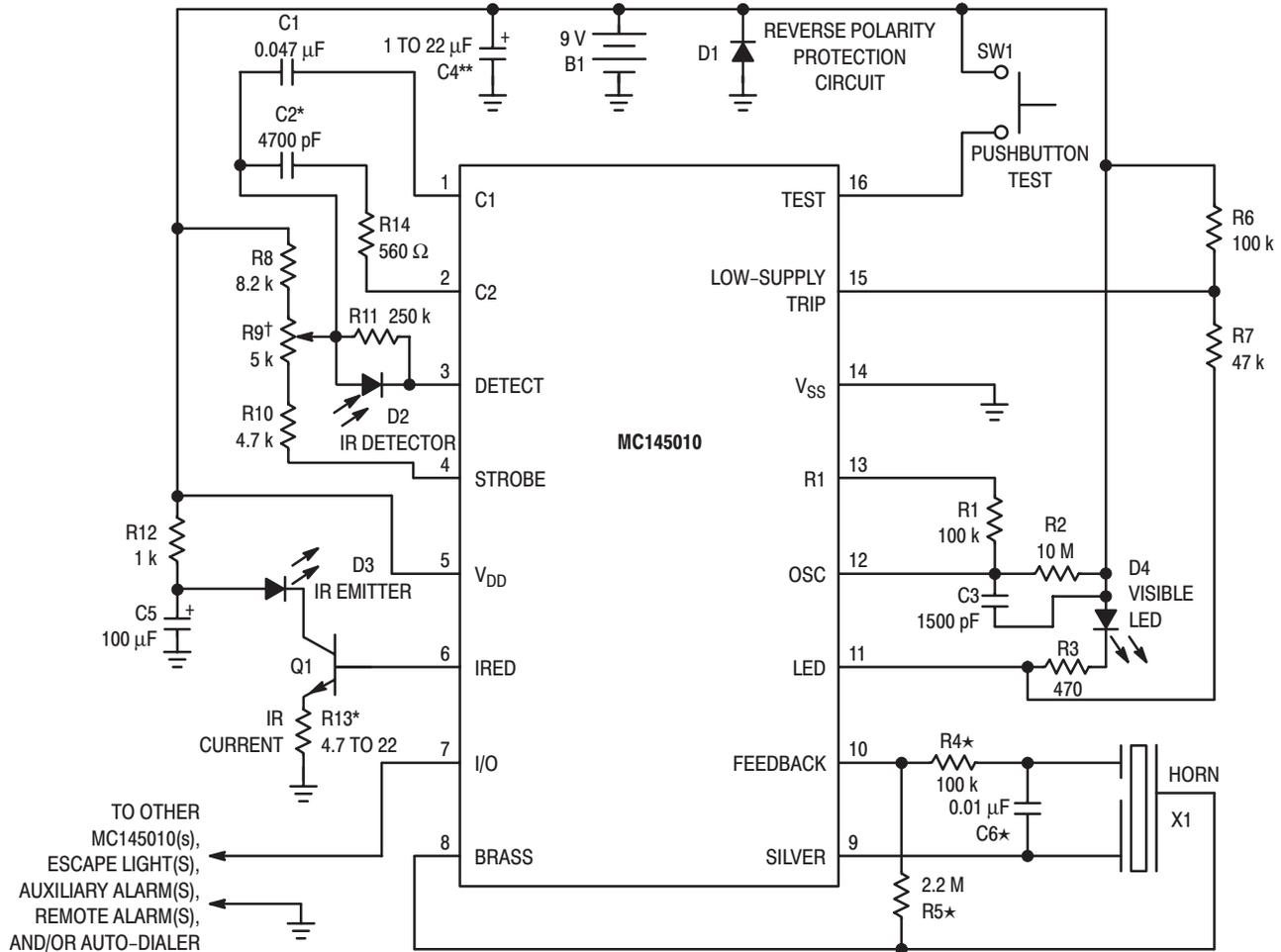
\*Values for R4, R5, and C6 may differ depending on type of piezoelectric horn used.
