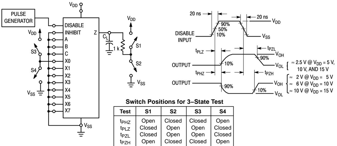
Figure 3. 3-State AC Test Circuit and Waveform
