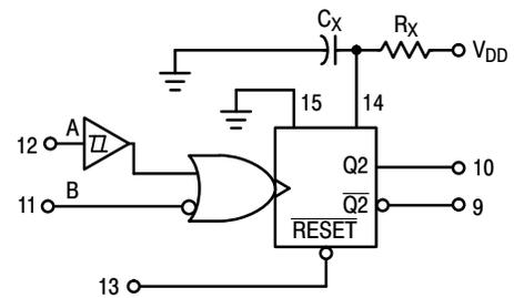
R<sub>X</sub> AND C<sub>X</sub> ARE EXTERNAL COMPONENTS.
