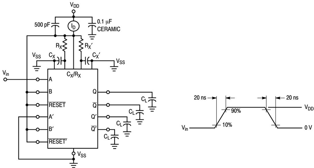
**Figure 2. Power Dissipation Test Circuit and Waveforms**
