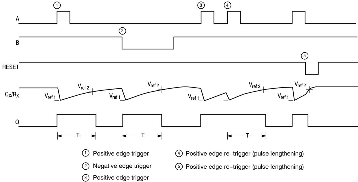
Figure 10. Timing Operation
