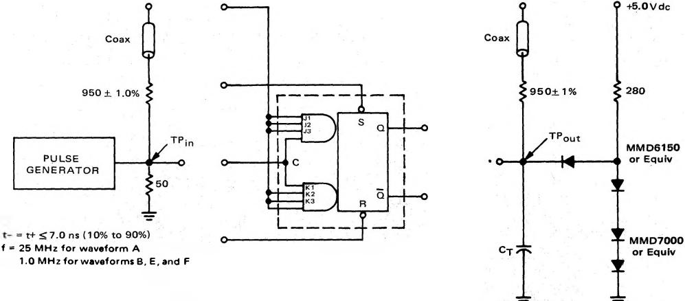
Two pulse generators are required and must be slaved together for testing SET and RESET. Only one pulse generator is required for J, K, and CLOCK tests.
