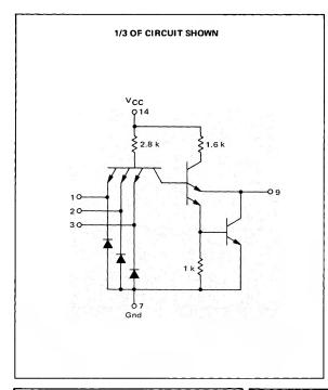
This device consists of three independent 3-input AND gates. The outputs of each gate are available as ORing nodes. Using the MC3019 expander, with the MC3031 expandable gate, up to six AND gates can be ORed together.
