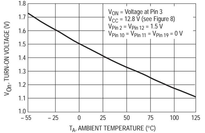
Figure 4. Reference Voltage versus Temperature
