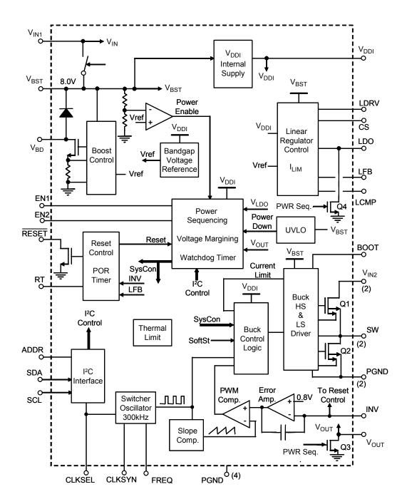
Figure 1. 33701 Simplified Block Diagram
