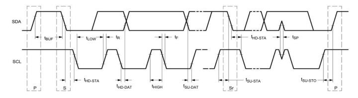
Figure 2. Definition of Time on the I<sup>2</sup>C Bus
